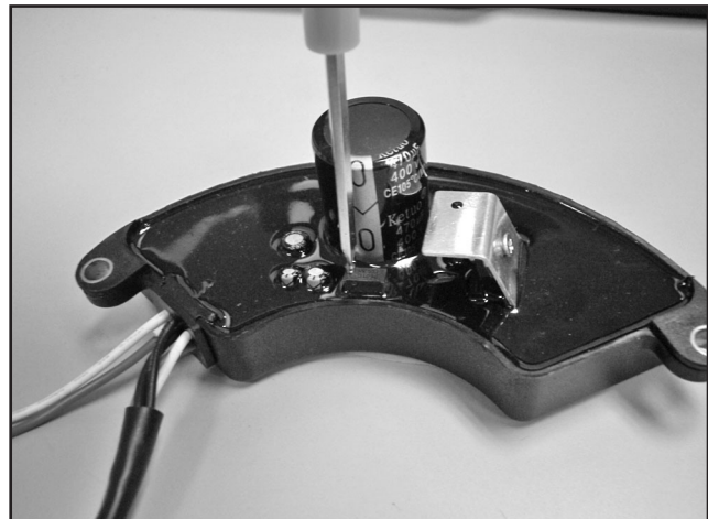
Figure 10. Voltage Regulator Adjustment Screw
